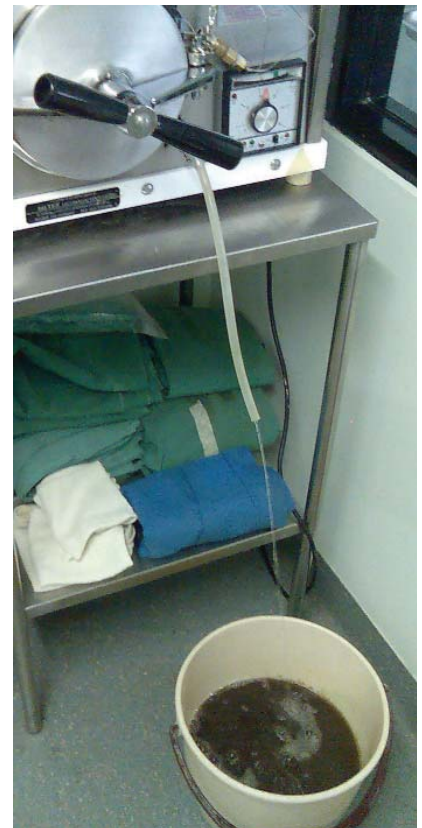
Figure 2. Classic example of the "brown water" syndrome. The water in the bucket was drained from the water reservoir of this steriliser. The build up of contamination that occurs when water is recycled is clearly visible.
