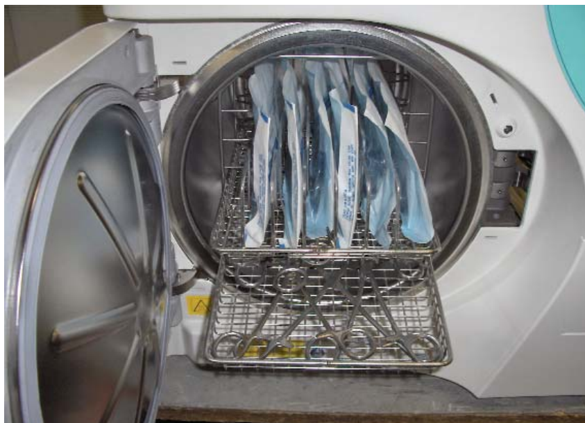
Figure 4. This illustrates a well-loaded steriliser. In this case, a vertical rack has been used for maximum sterilising and drying performance.
