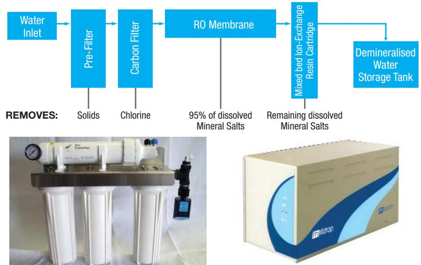
Figure 2. The process steps commonly used to produce high quality water suitable for use in a steriliser and examples of integrated Reverse Osmosis and Ion Exchange systems.
