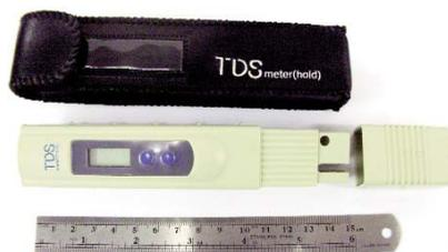
Figure 4. Convenient TDS Meters used to regularly check water quality for bench top sterilisers.
